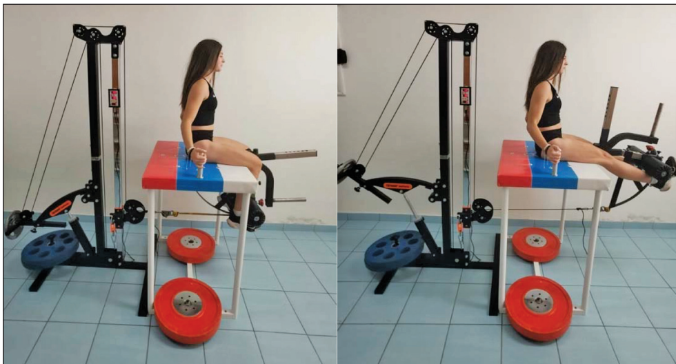
Figure 1. Position of the tested person on Iso+ Force2 when testing knee extension
