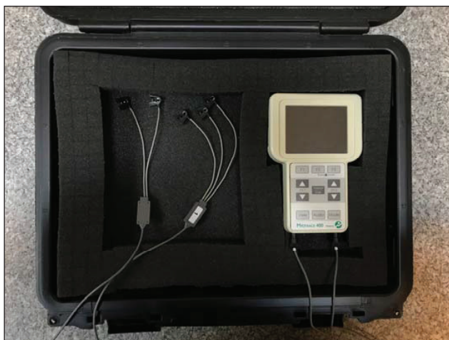
Figure 1. Surface electromyography (sEMG) system: Noraxon MyoTrace 400 (source: own materials)
